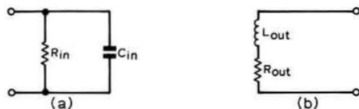
Fig 3. Equivalent circuits. (a) Input circuit, (b) output circuit
